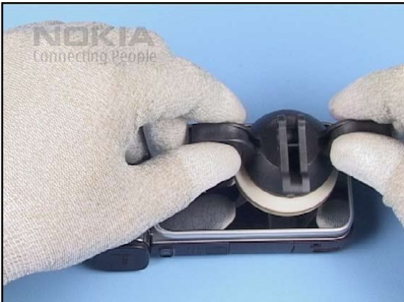
3. Position the SS-107 on the SUB LCD WINDOW as shown.
