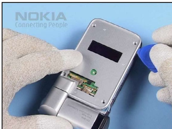
12. Slide the SRT-6 along the sides of the FLIP B-COVER to release all clips.
