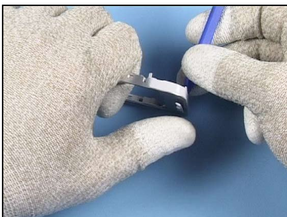
42. Remove the GRIP BUMPER by pushing it out from the inner side of the cover.
