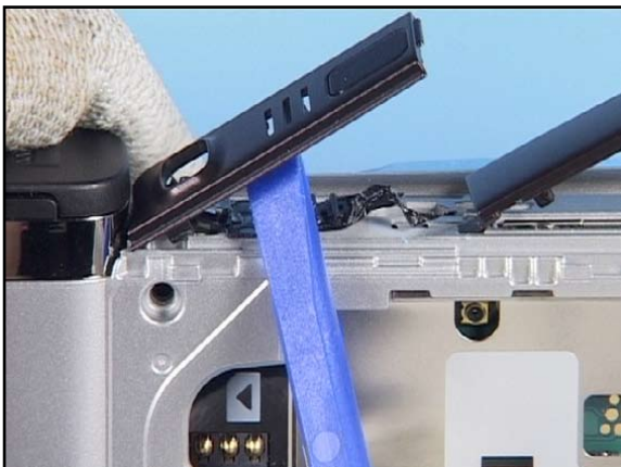
13. Use the SS-93 as a lever to unglue the ORNAMENT L ASSY (INCL. ADHESIVE). Do not reuse it.
