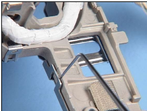
43. Unlock the SIM SHIELD COVER with the dental pick...
