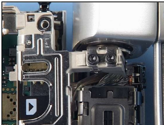
26. ...and gently separate the Upper Block from the Lower parts.
