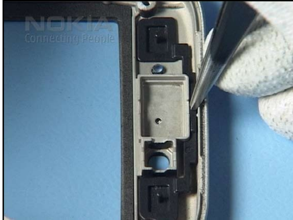
2. Carefully place the FLIP SOFT KEYMAT into its place.
