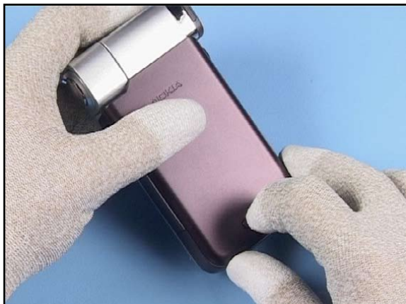
7. Unlock and remove the GRIP C-COVER.
