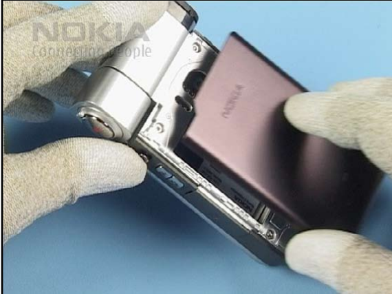
31. Finally fit the GRIP C-COVER ASSY.
