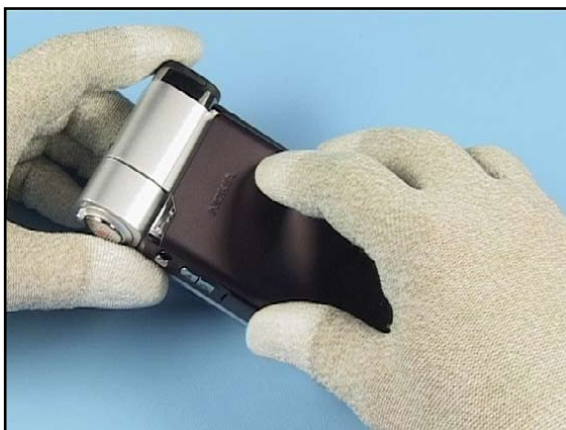
72. Finally fit the GRIP C-COVER ASSY.
