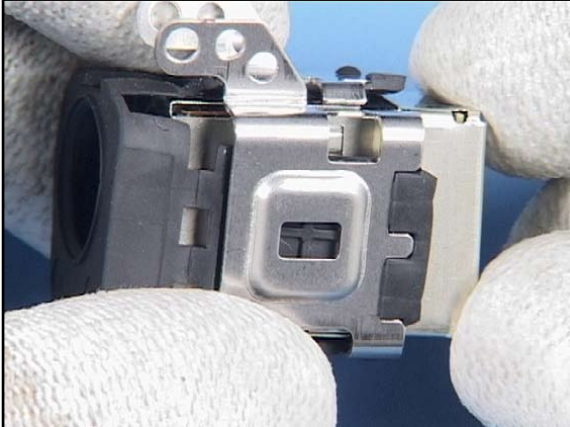
37. Insert the CAMERA MODULE into the FRAME.
