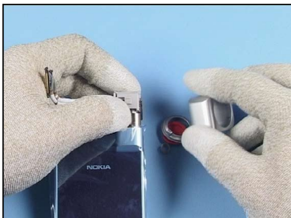
57. Remove the CAPTURE KEY BUTTON, ZOOM KEY LEVER and the CAPTURE RETURN SPRING.
