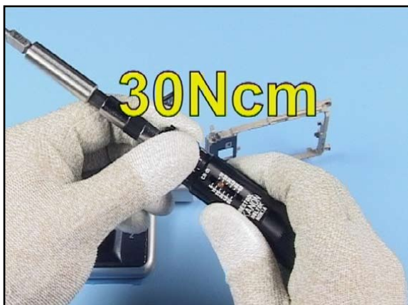
15. Set torque driver to the correct torque.
