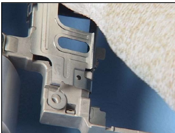
18. Fit the SIM SHIELD COVER.
