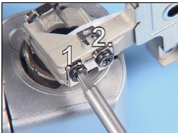
17. Tighten the SCREWS in the order shown.
