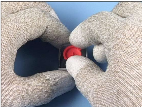
3. Place the CAPTURE KEY BUTTON in to its place.
