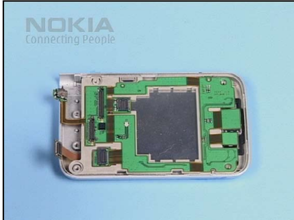
8. Gently turn the assembly as shown and ensure that the FLIP FRAM ASSY and the MAIN LCD are correctly placed onto the FLIP A-COVER.
