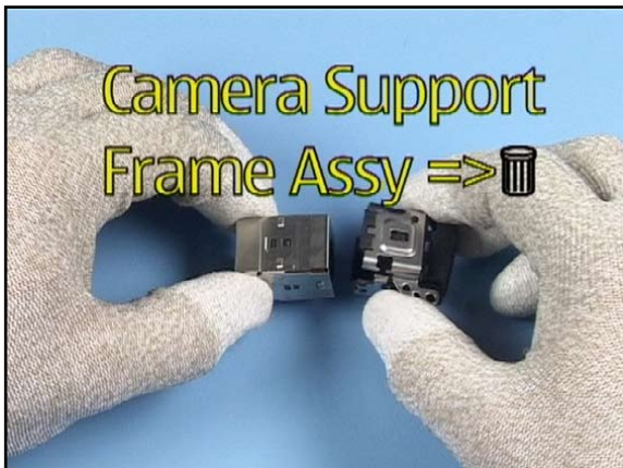
54. ...and separate the CAMERA MODULE from the SUPPORT FRAME ASSY. Do not reuse the CAMERA SUPPORT FRAME ASSY.
