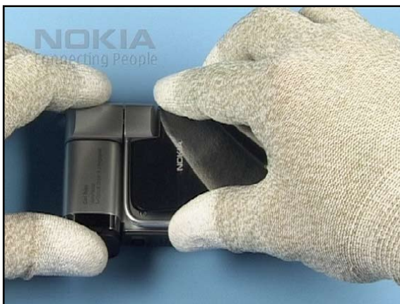
28. and align it exactly with the FLIP B-COVER.
