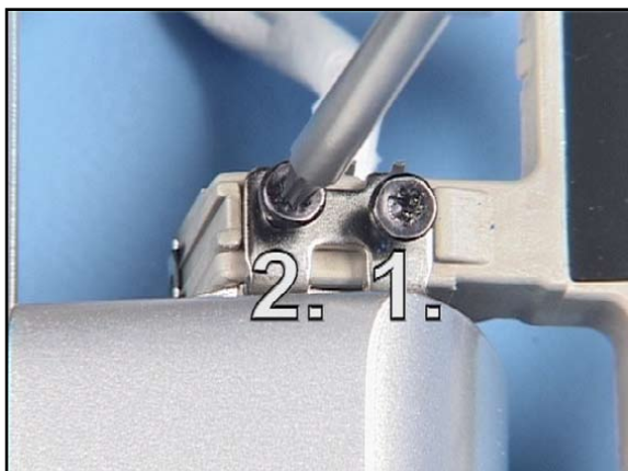
47. Undo the two Torx Plus size 6 screws in the order shown...
