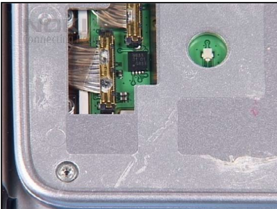
9. Only discard the FLIP B-COVER when the adhesive is gluing strongly and can not be removed completely.
