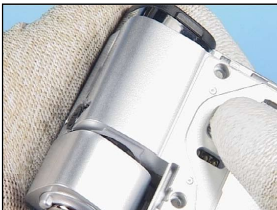
18. Unlock the last two snaps on the hinge side and remove the GRIP B-COVER.
