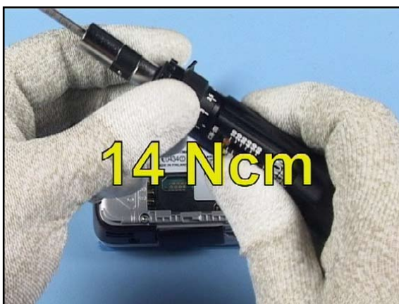
60. Set the torque driver to the correct torque.
