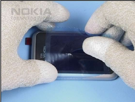
7. ...and cover the MAIN LCD with a protective film.
