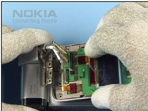
12. Align the FLIP A-COVER with the HINGE ASSEMBLY.
