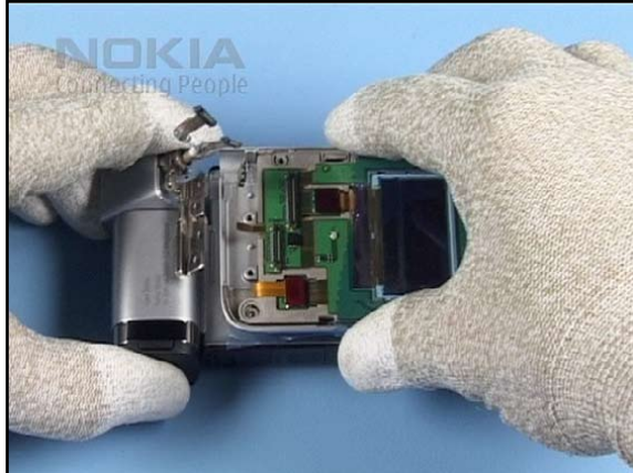
20. Open a bit the HINGE as shown and separate the upper parts from the LOWER BLOCK.
