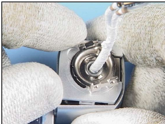
7. Fit the CAPTURE KEY INNER COVER as shown.
