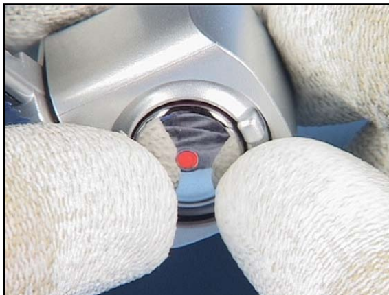
8. Now, check the correct position of the ZOOM KEY LEVER...
