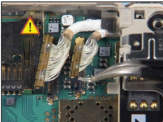
24. Place the tip of the tweezers exactly under the connector plug and carefully lever it up as shown.
