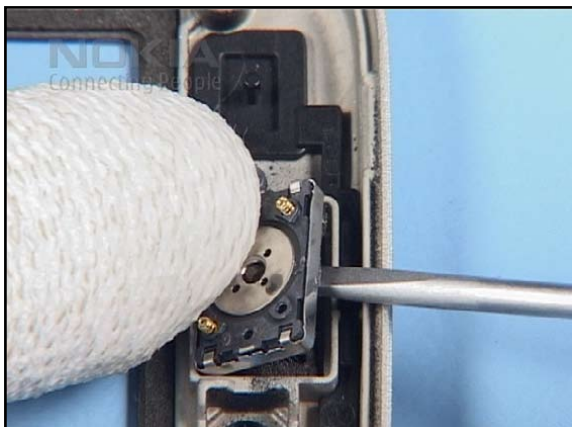
24. Now, lever the EARPIECE from its guidance...
