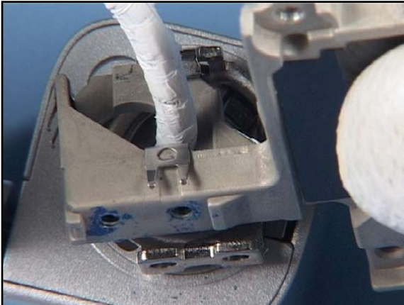
49. Gently separate the GRIP INNER FRAME from the UPPER BLOCK.
