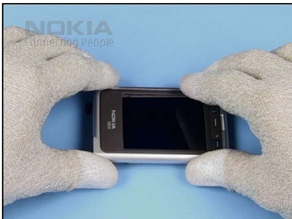
6. Align the FLIP A-COVER with the FLIP FRAME ASSY...
