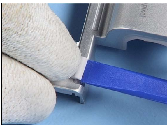
41. Remove the PILLOW with the SS-93.
