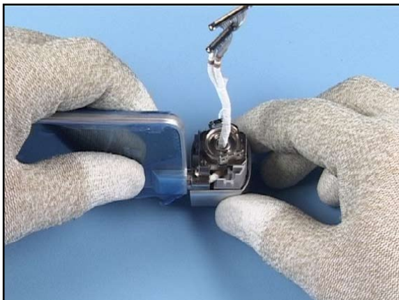
6. Carefully, press the HINGE ASSEMBLY into the CAPTURE KEY COVER.
