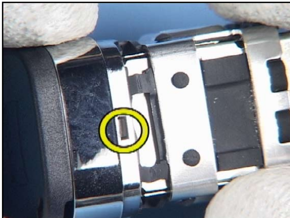
40. Ensure that the hooks hold well the CAMERA BEZEL.
