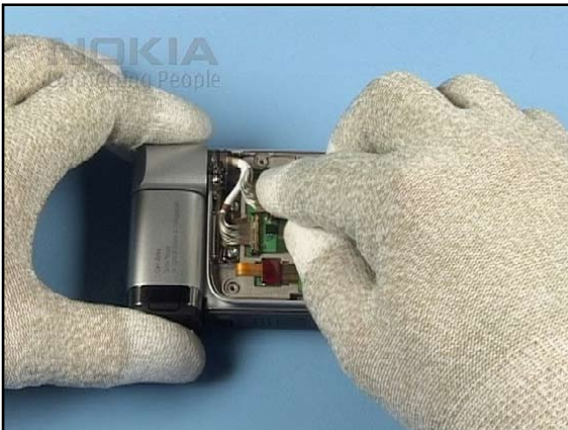
21. Very gently, close the both HINGE connectors.
