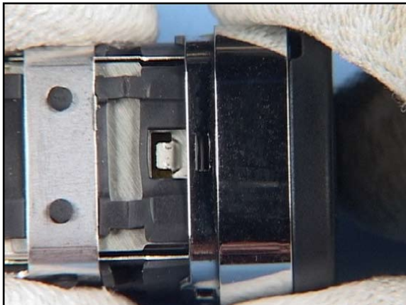
52. Pull out the CAMERA BEZEL with the LENS CUP ASSY from the CAMERA SUPPORT FRAME ASSY.
