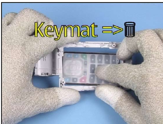
40. Separate the KEYMAT from the GRIP A-COVER and discard it.
