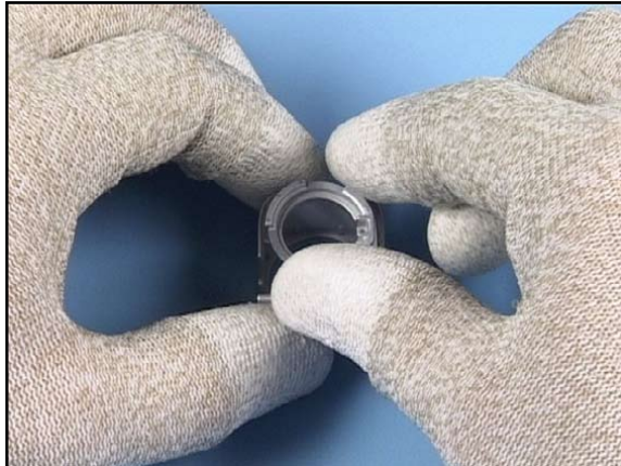
2. Place the ZOOM KEY LEVER PAINTED into the CAPTURE KEY COVER PAINTED as shown.
