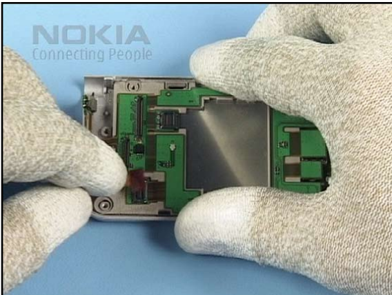
9. Close the MAIN LCD connector.
