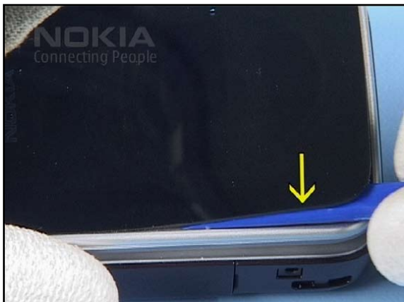
6. Place the SS-93 between the SUB LCD WINDOW and the FLIP B-COVER and separate the parts from each other.
