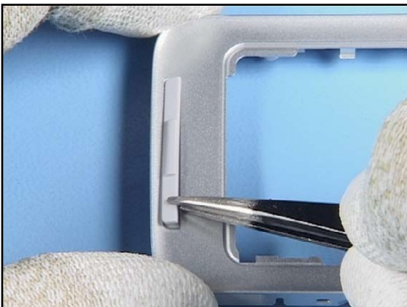
23. Fit a new GRIP BUMPER and secure it by pressing into place.
