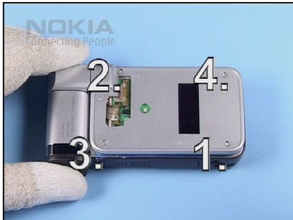
10. Undo the screws in the order shown...
