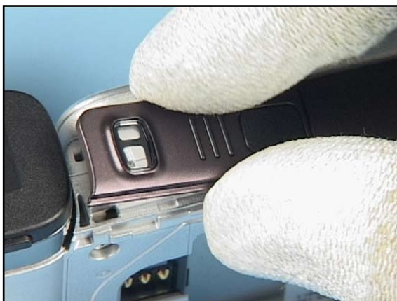
66. ...and fit the ORNAMENT L ASSY into its place.
