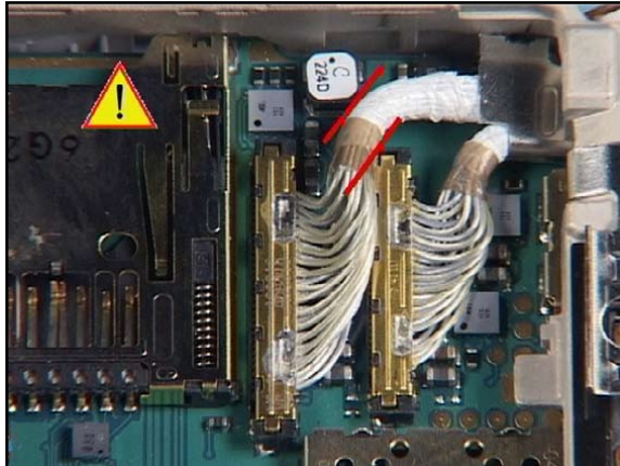
50. Ensure that the cable is positioned correctly to avoid squeezing it when assembling the LABEL PLATE.
