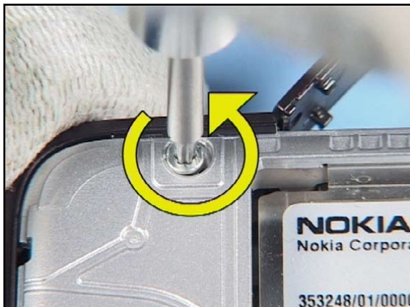
61. To prevent damaging the plastic threads, first turn the screws to the left...
