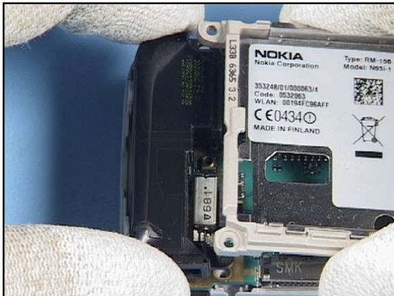
52. Lift the GRIP INNER FRAME a bit and gently place the ANTENNA into its position.
