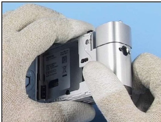
56. First close the snaps on the hinge side.
