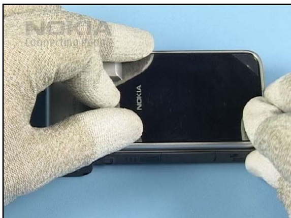
29. Secure the window by pressing it into the FLIP B-COVER.
