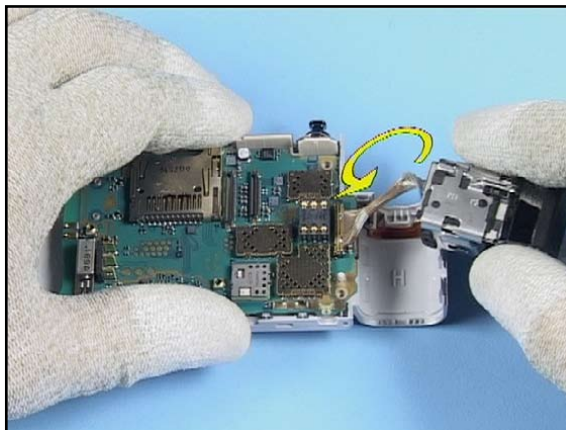
44. Turn the CAMERA MODULE as shown...
