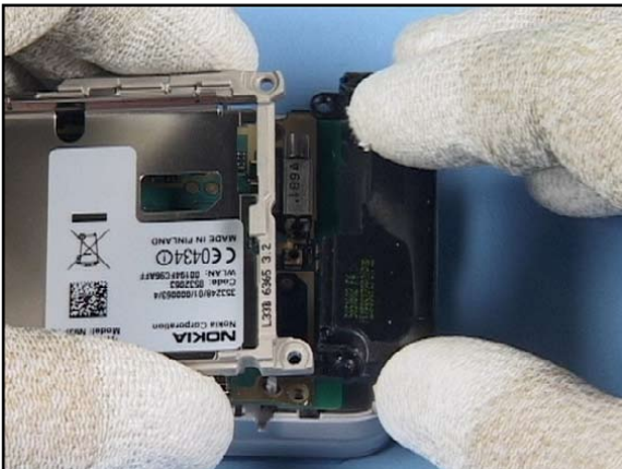
21. Lift the GRIP INNER FRAME a bit and remove the ANTENNA ASSY.
