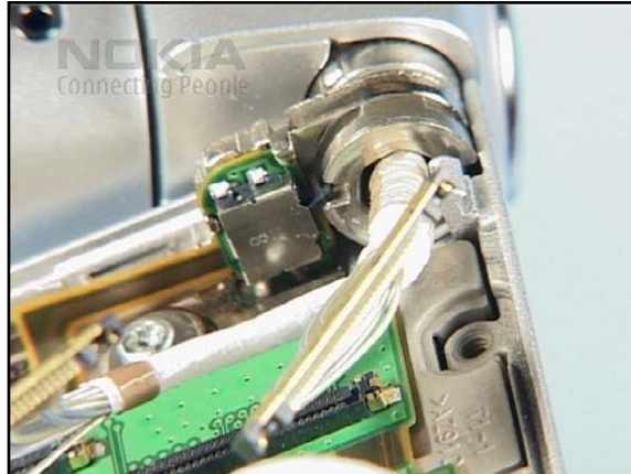
20. ...and check the functionality of the switch by turning the FLIP A-COVER to both directions.
