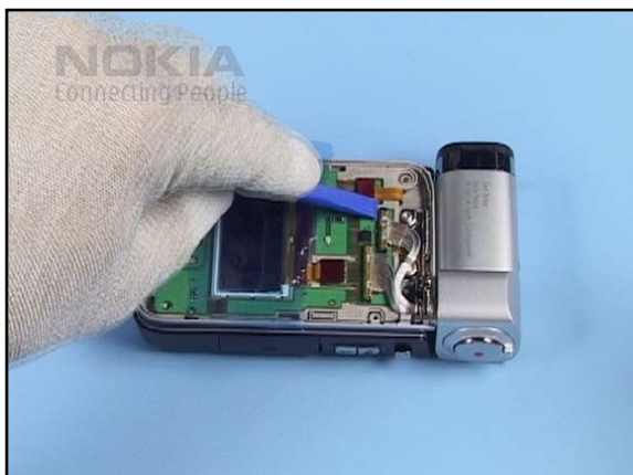
15. Use the SS-93 as a support when opening the HINGE connectors.
