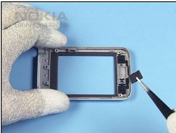
3. Always use a new EARPIECE GASKET when replacing the EARPIECE.
