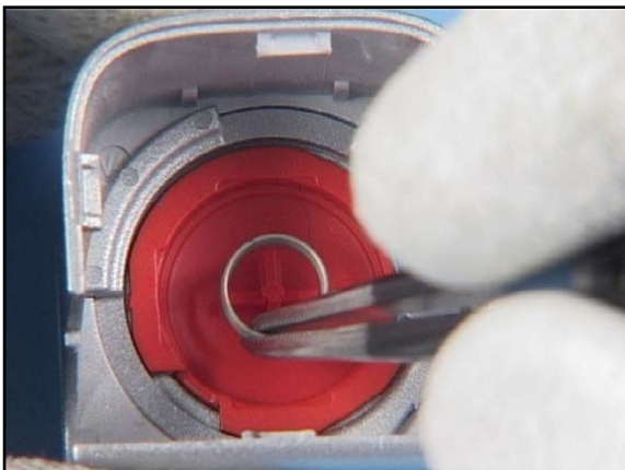
5. Place the CAPTURE RETURN SPRING in to its place.
