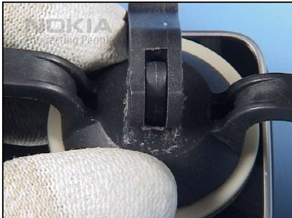
4. Press down the lever to create vacuum in the cup.
