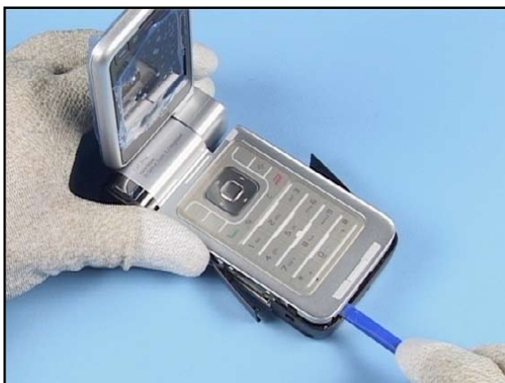
16. Unlock all snaps of the GRIP B-COVER.
