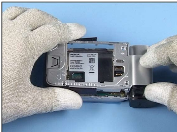
55. Align the GRIP B-COVER with the GRIP A-COVER.
