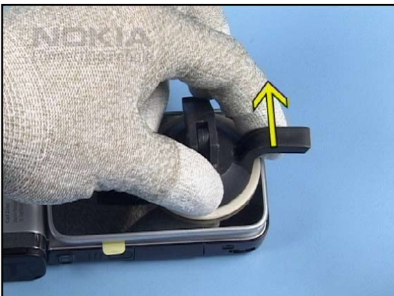
5. Carefully, pull at the grip to lift a bit the SUB LCD WINDOW.
