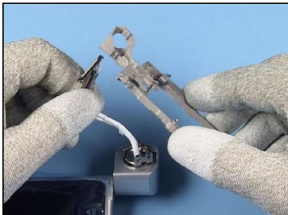
13. Feed the HINGE cables into the opening of the GRIP INNER FRAME.
