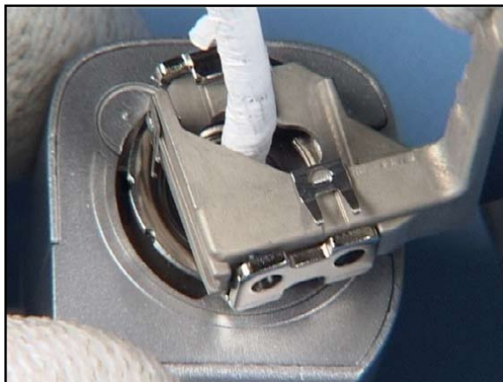
14. Position the GRIP INNER FRAME onto the HINGE ASSEMBLY.
