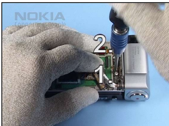
17. Undo the screws in the order shown...
