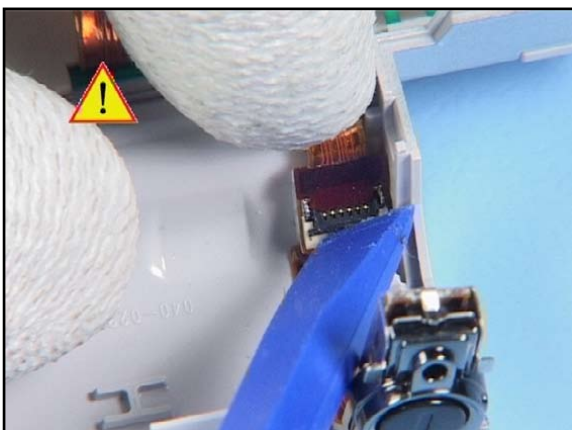
27. Very gently, close the connector with the SS-93.
