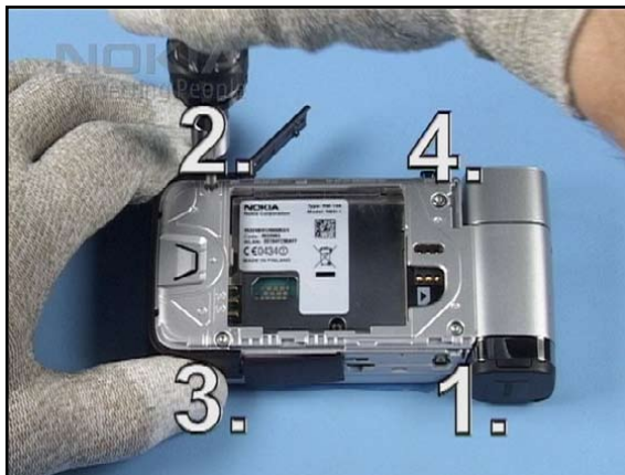
62. ... and then tighten them to the correct torque in the order shown.
