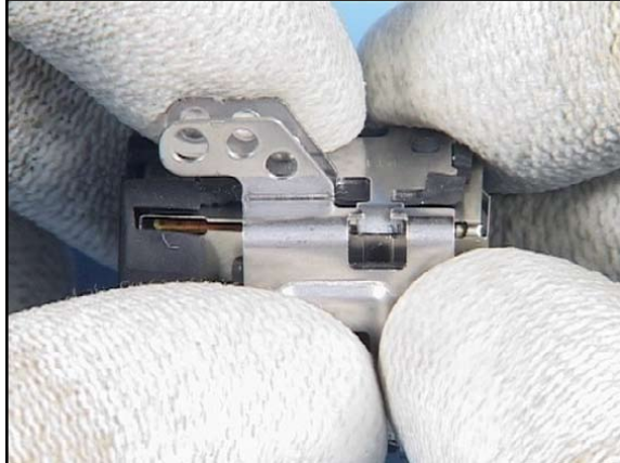
38. Squeeze the CAMERA SUPPORT FRAME ASSY until it close.
