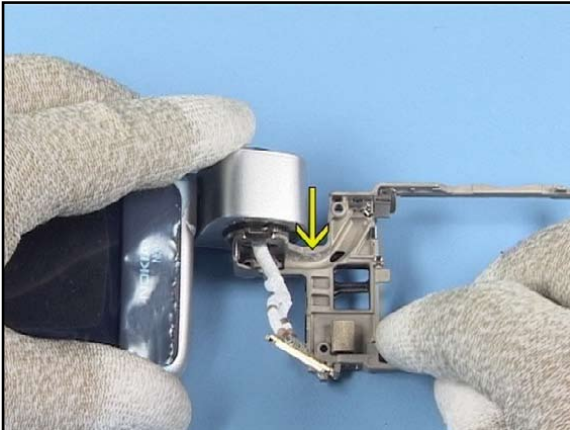
19. Ensure that the adhesive is glued into the shown place.
