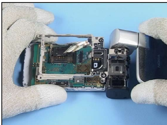
47. Align the GRIP INNER FRAME with the GRIP A-COVER avoiding squeezing the CABLE ASSY.
