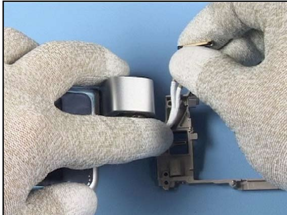
20. Place the HINGE cables into the guide of the GRIP INNER FRAME.
