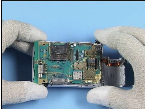
32. Turn the ENGINE MODULE as shown and align it with the GRIP A-COVER.
