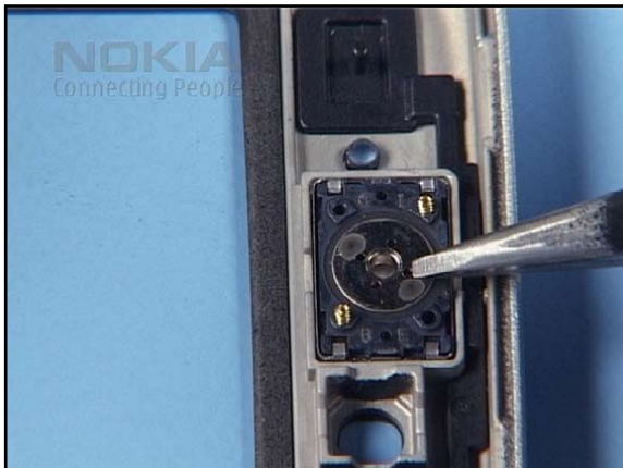
4. Mind the spring contacts while handling the EARPIECE.
