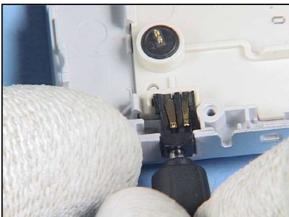
29. Fit the DC-JACK with the DC-plug.
