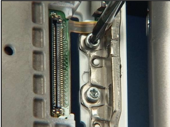
31. Unscrew both torx size 6 screws and discard them.
