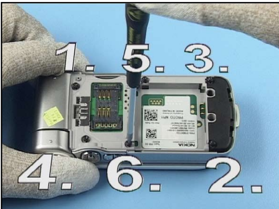
9. Remove the six torx plus size 6 screws in the order shown.
