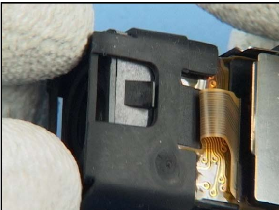
15. Shift the Camera Cushion into its correct position.
