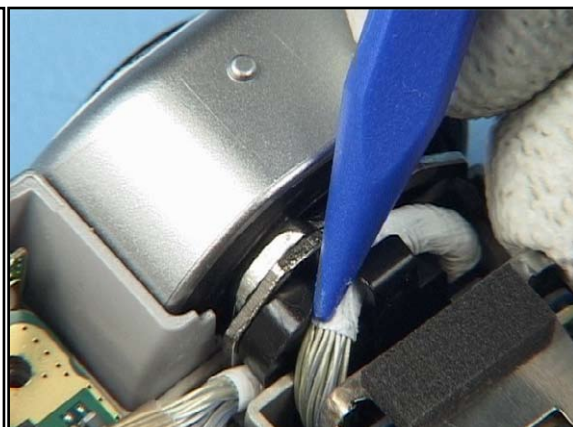
18. Ensure the correct positioning of the cables while placing the Camera Module into its housing.
