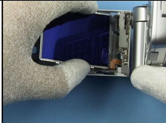
20. Remove the protection film from the Main Display. Slot the flex foil through the Flip B-Cover.
