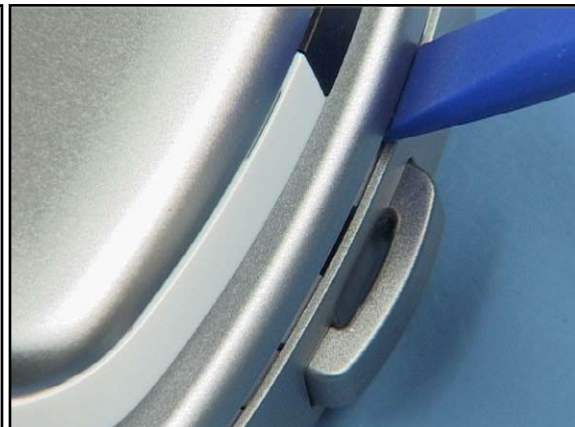
10. Carefully pry open the snaps of the Grip A-Cover with the SS-93.
