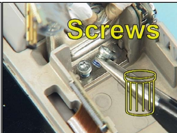
36. Always use new screws when reassemble.
