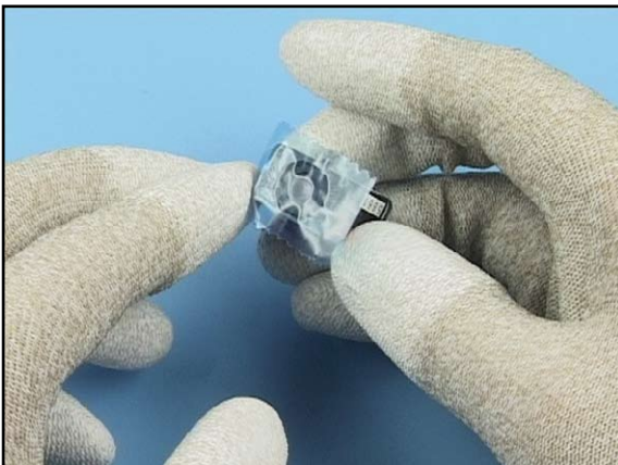
27. Cover the lens with a plastic film.
