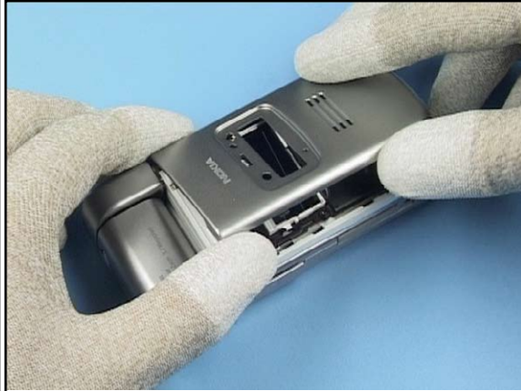
8. Remove the Flip C-Cover assembly.
