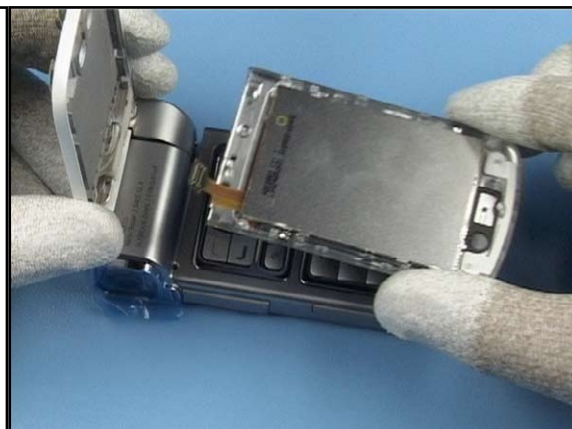
24. Push out the Flip A-Cover together with the Main Display.
