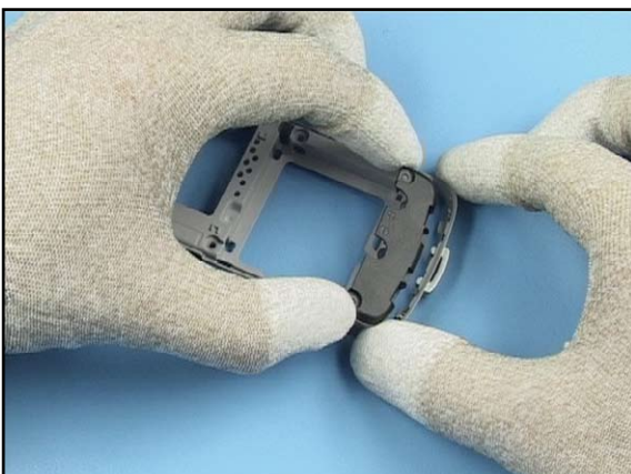
23. Click the Antenna Cover into its place.
