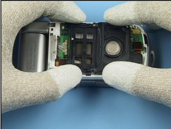
36. Place the Flip Frame, mind the correct positioning.
