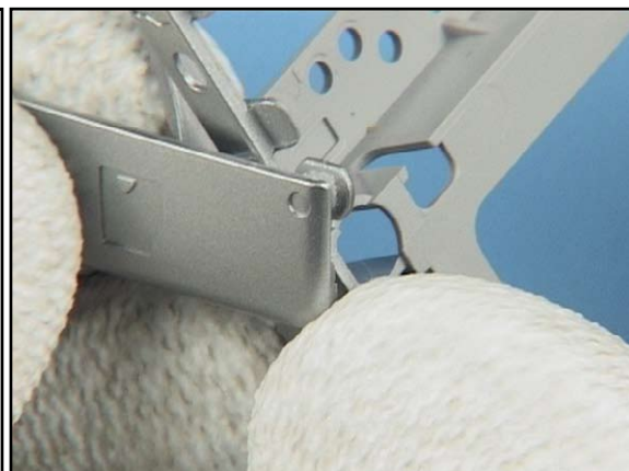
12. Push out the SD Bung Painted.
