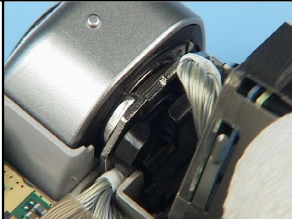
20. Carefully lift out the Camera unit, mind that the coax cables are still connected.
