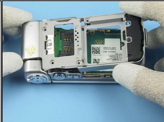
26. Position the Grip B-Cover over the Assembly.
