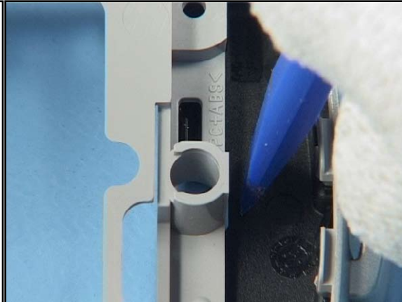
14. Hold down the Antenna Cover while lifting the Grip B-Cover.
