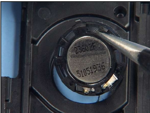
15. Lift out the glued in IHF Slim.
