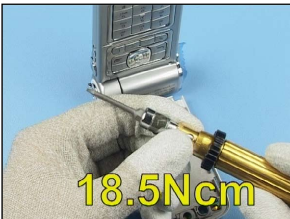
11. Fit the torx size 6 bit and set the correct torque.
