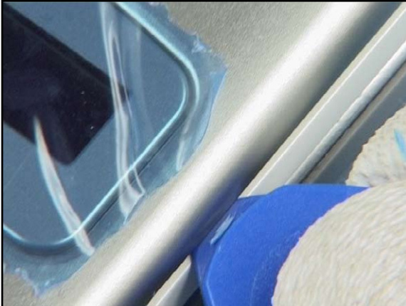
7. Slide along the sides of the Flip C-Cover Assembly, open the two clips as shown.
