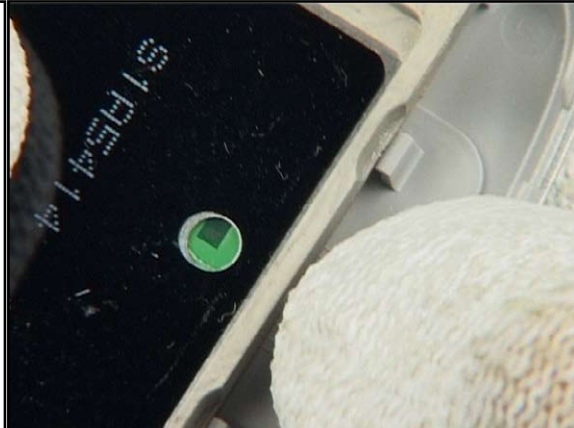
38. Unlock the snaps of the Grip A-Cover and separate the parts.
