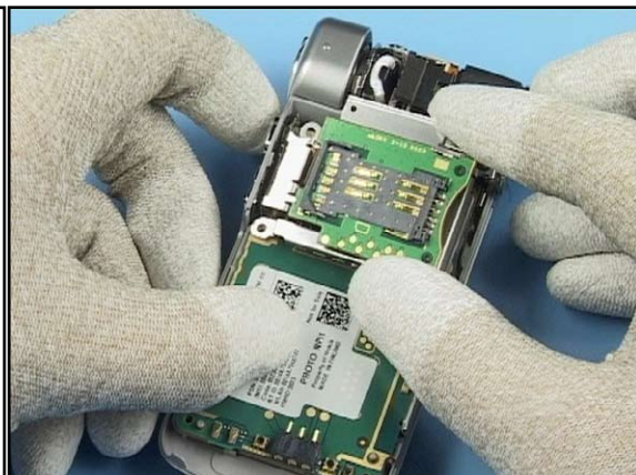
22. Place the SDSIM PWB Module and click the latches into their places.
