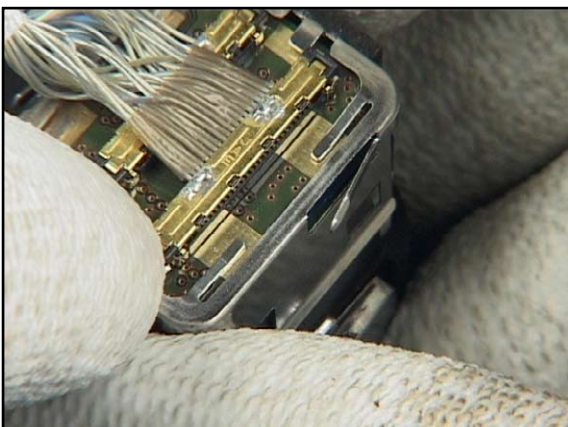
17. Now connect the Camera Module. Mind the correct positioning of the connectors.
