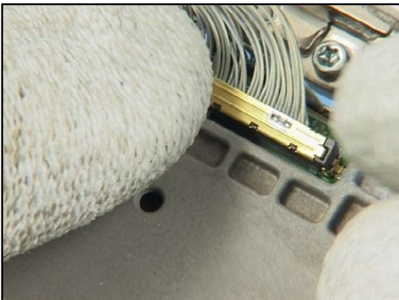
15. Close the connector while pushing from behind the Flip PWB Module.
