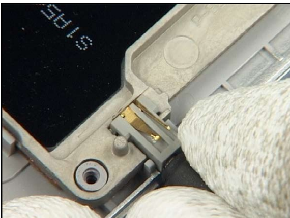
9. Place the DC Jack into its compartment.
