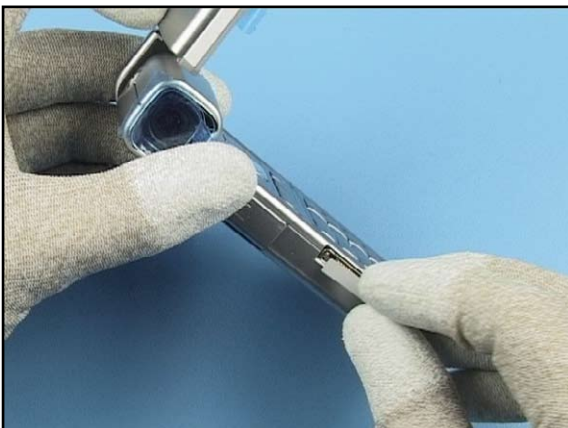
39. Complete the Assembly with the POP Port Bung Painted.
