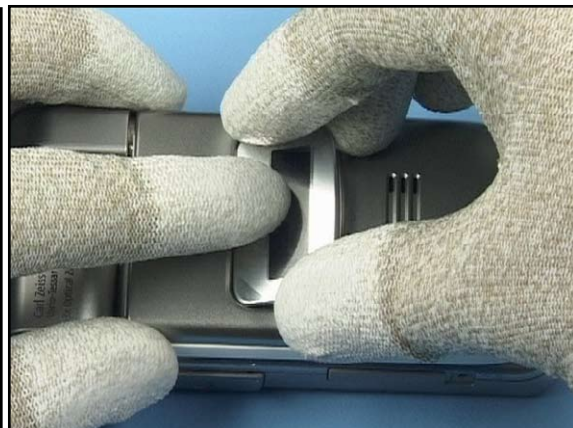
47. Place a new Sub Display Window, smooth it down evenly.
