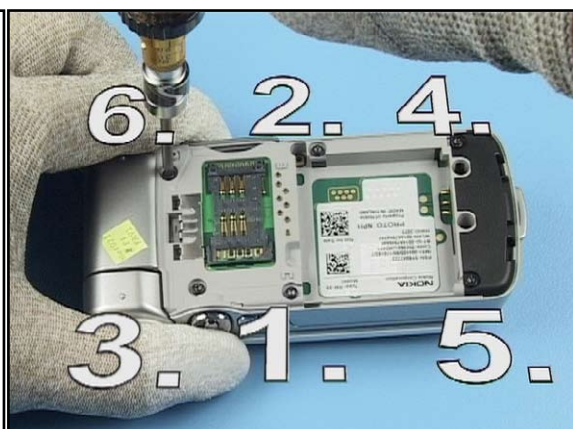
30. Then tighten them in the correct order shown.
