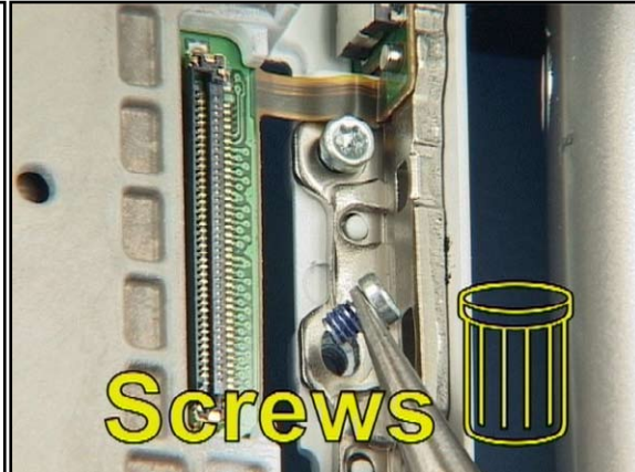
32. Always use new screws when reassemble.
