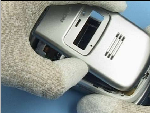
42. Place the Flip C-Cover, beginning from the top.
