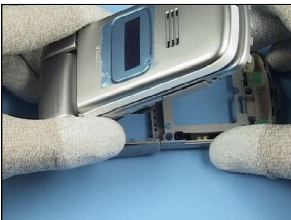
11. Separate the Grip B-Cover.
