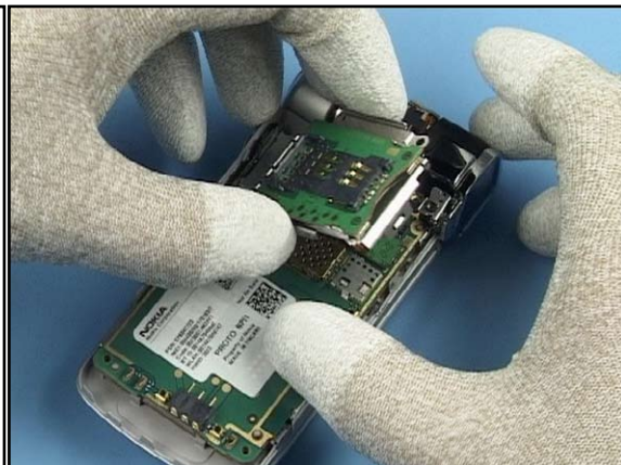
16. Lift up the SDSIM PWB Module.
