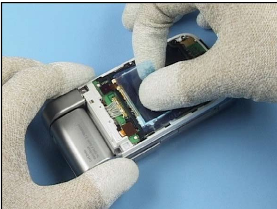
9. Protect the Sub Display with a plastic film.
