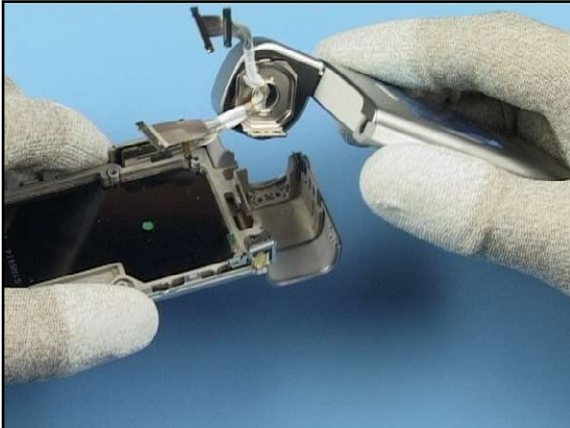
37. Bring the unit into position shown and separate the parts.
