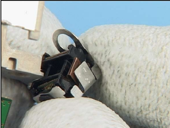
1. Place the Mic Clip, do not touch the microphones.
