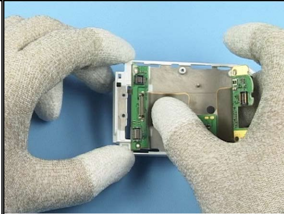
8. Align the Flip PWB Module to the guides and smooth it down evenly.
