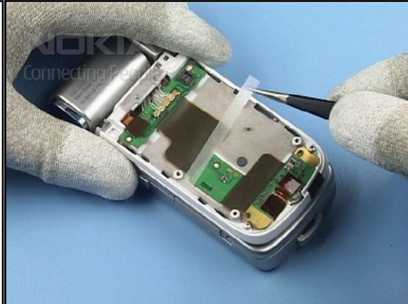
32. Stick a new Flip Frame Adhesive Tape. Smooth it down evenly and remove the protection film.
