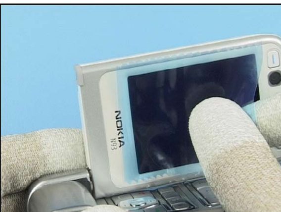
46. Cover the Main Display with a plastic film.
