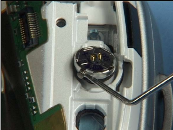
19. Now the glued in Earpiece can be removed easily.
