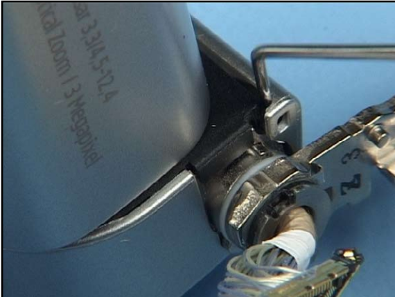
37. Release the latches of the Capture Key Cover Module.
