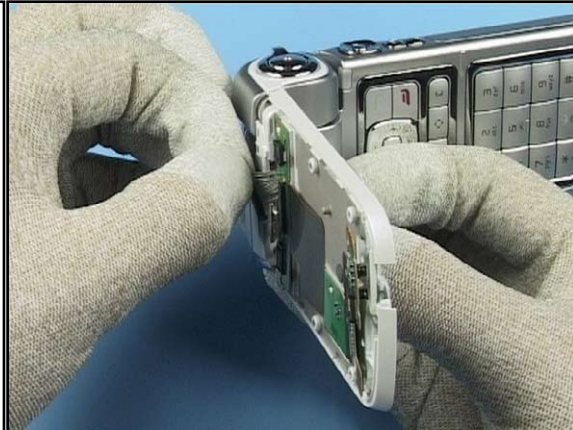
14. Slot the smaller connector through the Flip B-Cover.
