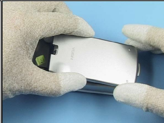
32. Place the Grip C-Cover Assembly, beginning from the bottom.
