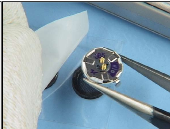
28. Always use a new Gasket when replacing the Earpiece.
