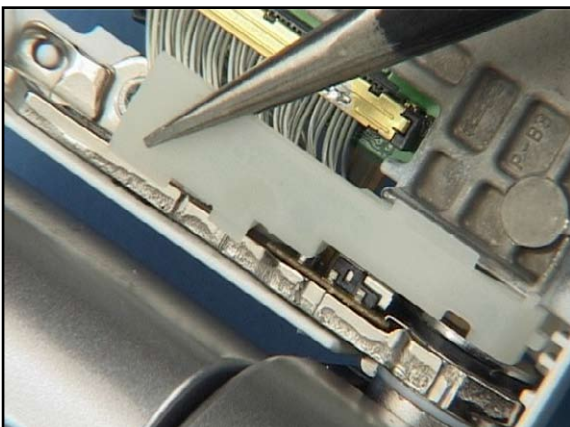
29. Mind the cables while removing the Detector Holder with tweezers.
