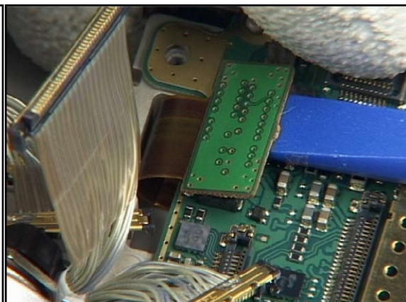
30. Disconnect the flex foil connector evenly.
