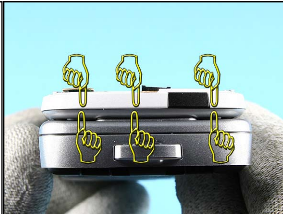
26. Check if there is no gap remaining between Flip A-Cover Assy and Flip B-Cover.
