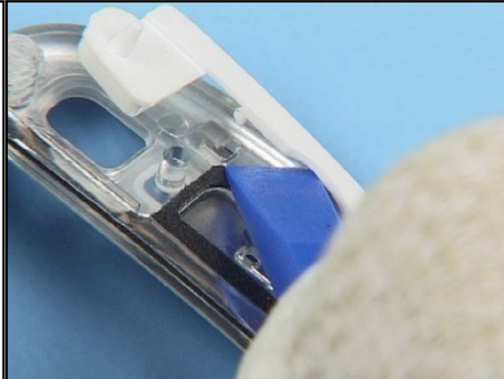
26. Carefully lever out the Flip Soft Keymat.
