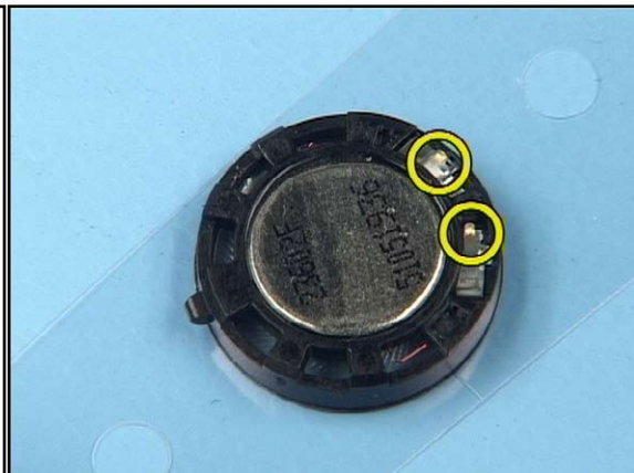
33. Mind the spring contacts while handling the IHF Speaker.
