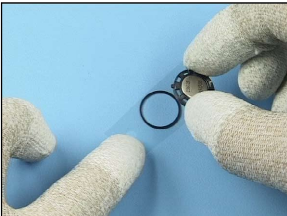
32. Use a new Gasket when replacing the IHF Speaker.
