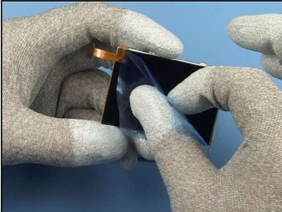
25. Protect the display with a plastic film.
