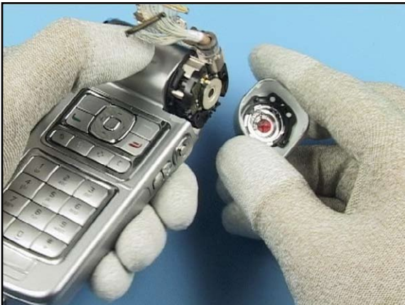
39. Now the Capture Key Cover Module can be removed easily.
