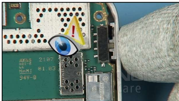
10. Check the functionality of the switch before going on.
