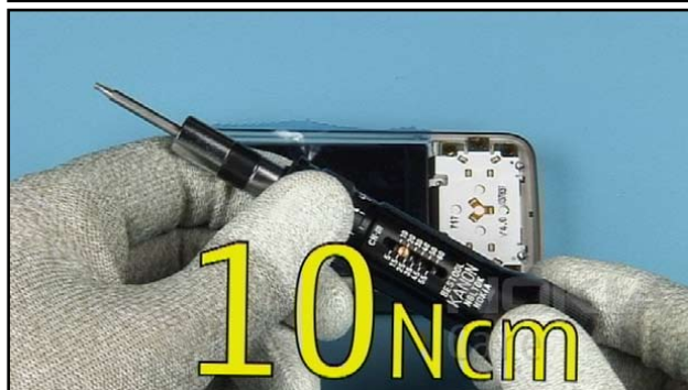
23. Set the correct torque.
