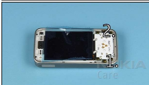
24. Tighten the screws in the order shown.
