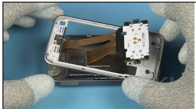
30. Use the A-COVER as support when turning the assembly.
