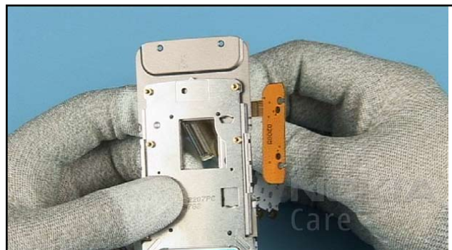
36. Slot the FLEX trough the recess of the SLIDE MODULE ASSY.
