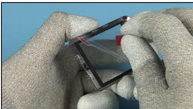
25. Remove the protective film from the WINDOW.
