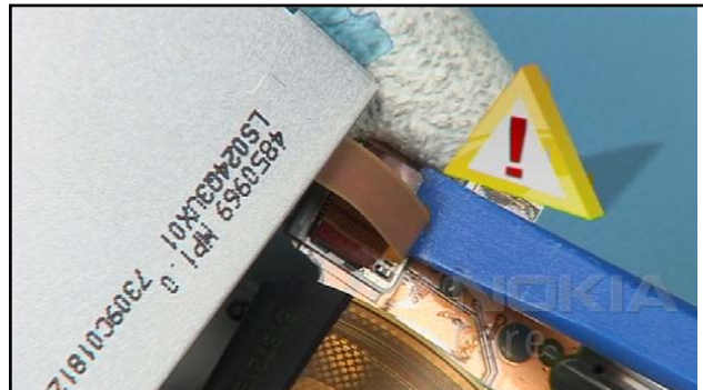
22. Open the flex connector of the LCD.
