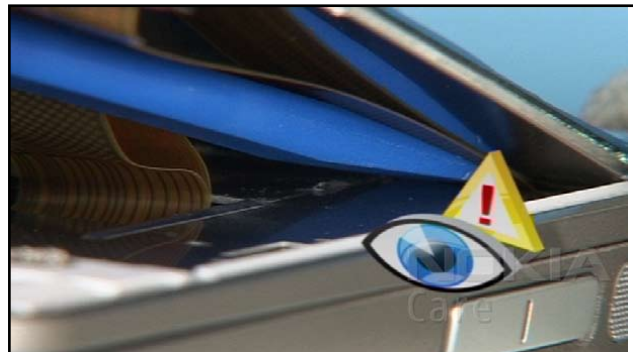
20. Note the correct positioning of the SS-93. Do not destroy the components underneath.
