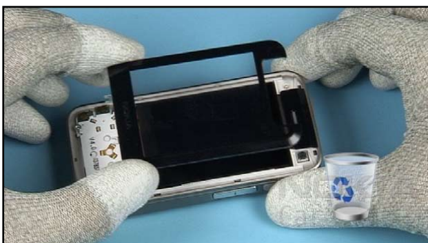
13. Now the WINDOW-ASSY can be removed. Do not use it again.
