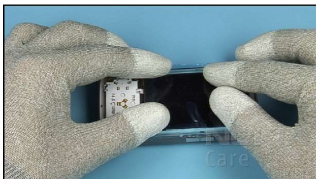
18. Place the LCD correctly.
