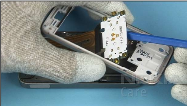
33. Now the A-COVER can be removed again.
