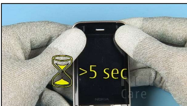
27. Push down the WINDOW, at least 5 seconds each 2 cm, beginning from the top in order to activate the adhesive coating.
