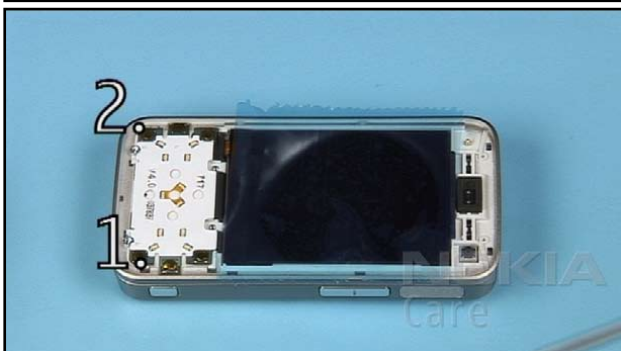
15. Unscrew the next 2 Torx size 6 screws in the shown order.
