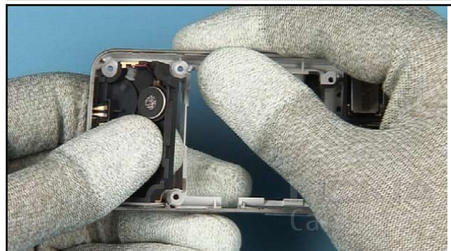
40. Push out the ANTENNA ASSY.
