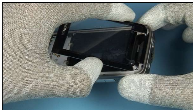
26. Insert the WINDOW, beginning from the top.
