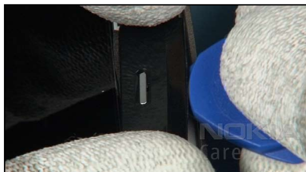
14. Lever out the GAMING KEY ASSY.
