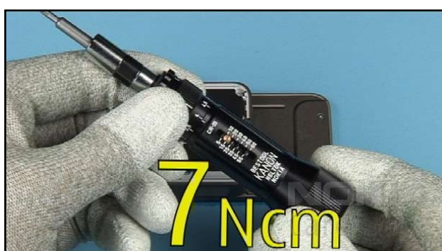
20. Set the correct torque.
