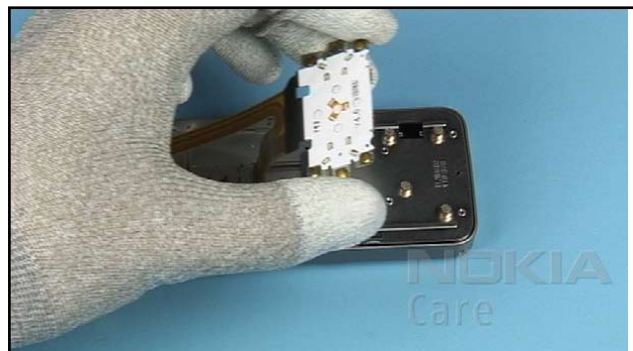
28. Gently lever out the EARPIECE. Prevent destroying the delicate clips of the A-COVER.
