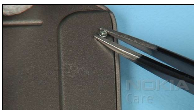
19. Insert these counter sunk screws.
