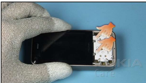
9. Unscrew these 2 Torx plus size 6 screws.
