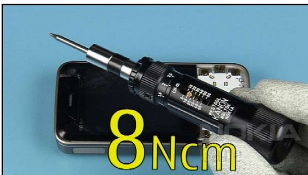
29. Set the correct torque.
