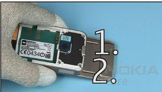
23. Release both countersunk screws in the order shown.
