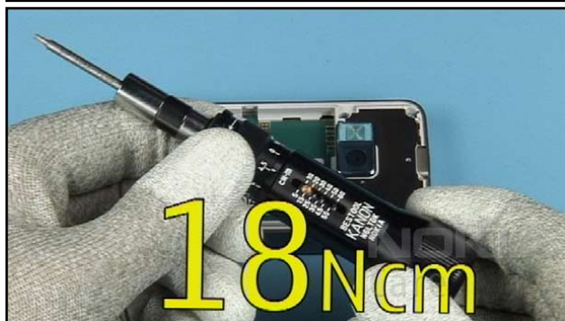
16. Set the correct torque.
