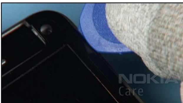
11. Release the adhesive of the WINDOW-ASSY with the SRT-6...
