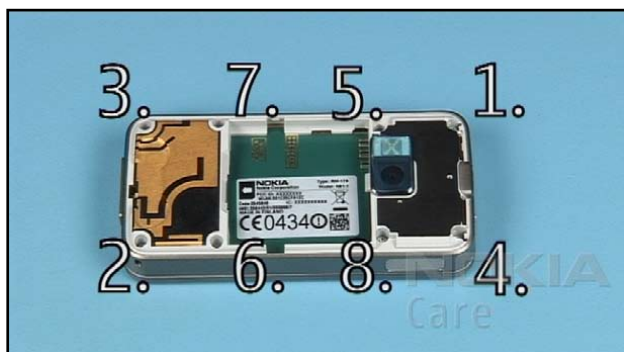
17. Tighten the screws in the order shown.
