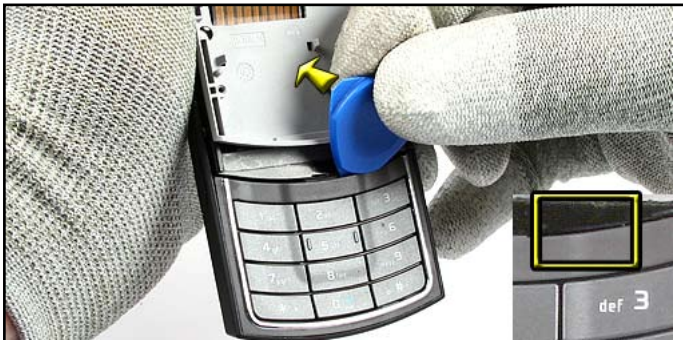
28. First start to unlock the first snap and then follow the shown order in picture 29.
