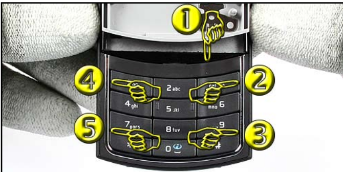
29. To unlock the KEYMAT BEZEL use the SRT-6 to open the 5 snaps in the shown order and at the correct place.
