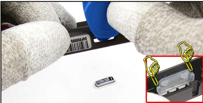
51. Push out the CAMERA KEY. Mind the correct assembling of the CAMERA KEY (small picture).
