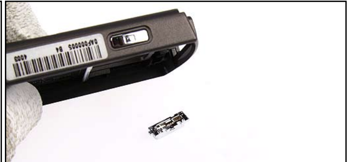
50. The C-COVER CATCH drops out easily.
