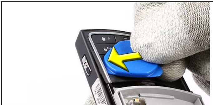
30. To open the snaps 2-5 only stick in the SRT-6 between ITU KEYMAT and KEYMAT BEZEL in the shown angle.
