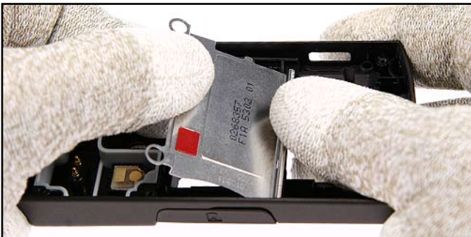
53. Gently, remove the BATTERY BASE ASSY.
