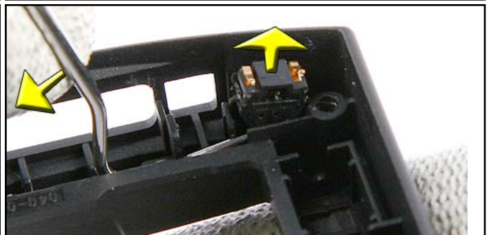
48. Use the dental tool to remove the MICROPHONE.
