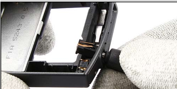
47. Use the DC-Plug to remove the DC-JACK.
