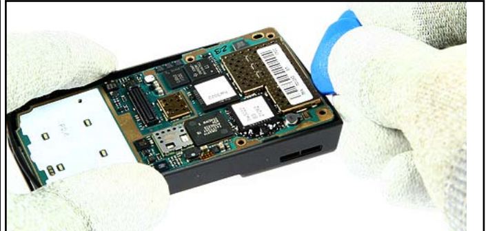
42. Lift up the ENGINE MODULE a bit, and remove it.
