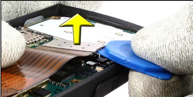
41. Open the FLEX I connector carefully.
