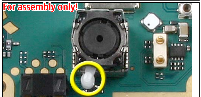
44. ... the camera macro lever of the 3MP CAMERA on the ENGINE MODULE.
