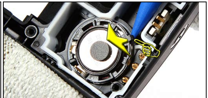
56. Lift up the IHF SPEAKER a bit, and remove it. Note the guide pin when re-assembling the IHF SPEAKER.
