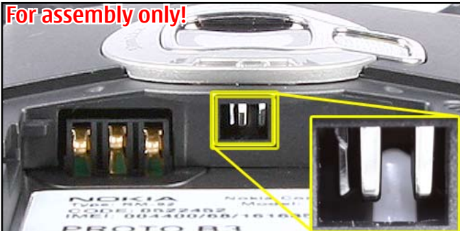
45. Note! After placing the ENGINE MODULE into the B-COVER ASSY check the window inside the battery housing if the CAMERA MACRO KEY and camera macro lever correct fit together.
