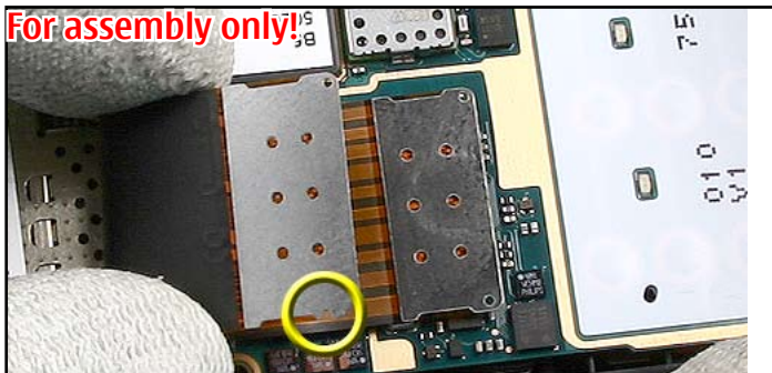
40. Mind the correct assembling when connecting the FLEX I/CONN MODULE to the ENGINE MODULE.
