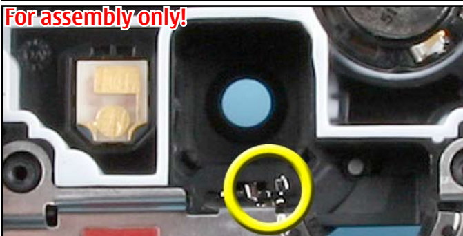
43. Note! For assembling ensure the correct position of the CAMERA MACRO KEY in the B-COVER ASSY and ...
