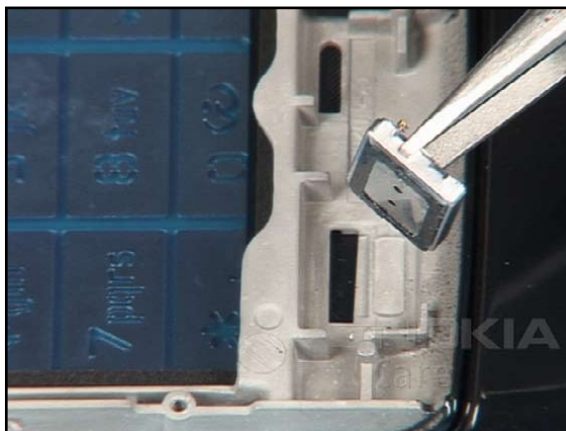
2. Fit a new gasket to the EARPIECE.
