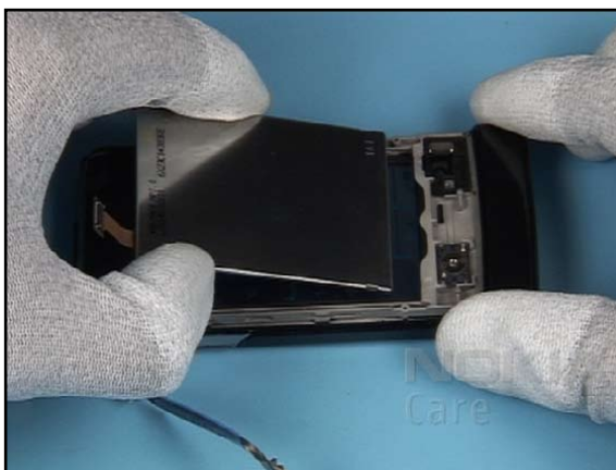
4. Remove the protection film and place the LCD.
