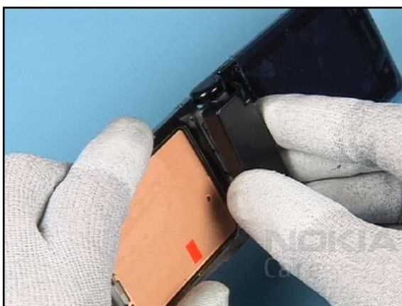
12. Place the HINGE COVER TOP. Mind the hooks!
