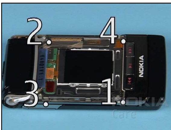
18. Apply the torque to the screws in the order shown.
