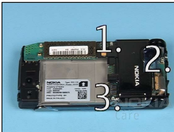
26. Tighten the screws in the shown order.
