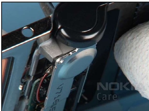
7. Bring the upper and lower block into position as shown.
