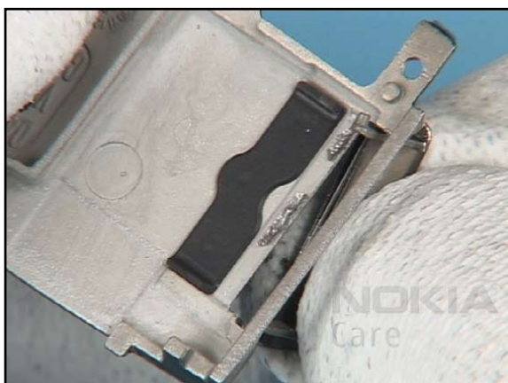
21. Insert the SD CARD DOOR as shown.
