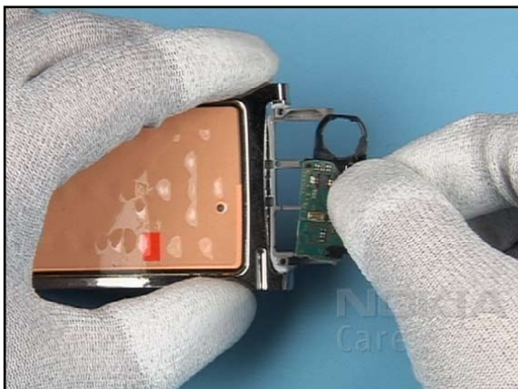
30. Remove the CAMERA PWB ASSEMBLY.
