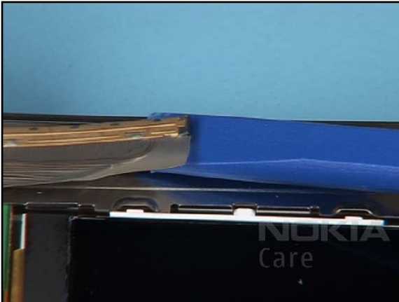
13. Carefully release the connector as shown. Avoid bending the connector.
