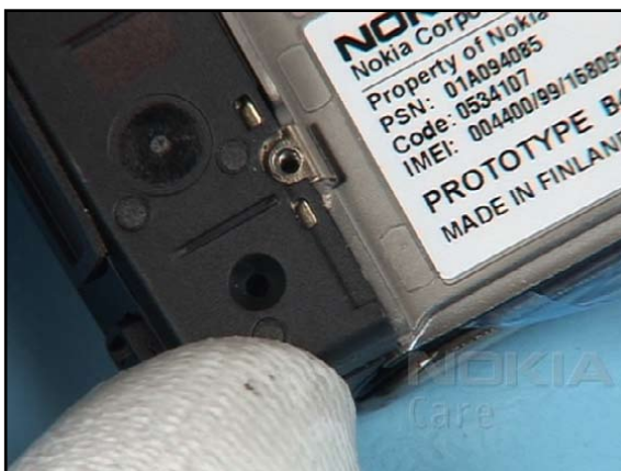
18. Place the ANTENNA MODULE. Mind the guides.
