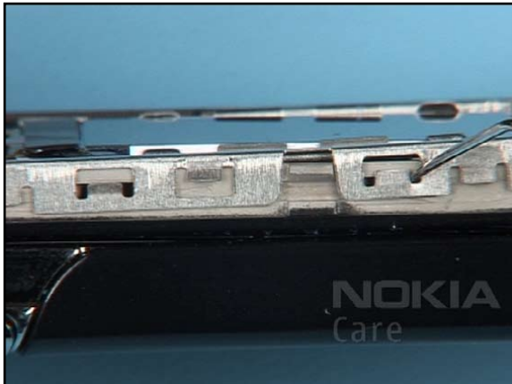
16. Open these 2 metal latches. Do not over bend these clips.
