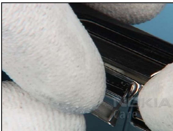
10. Open the SD DOOR. Carefully lever up and hold the D-COVER into position shown with your fingers.
