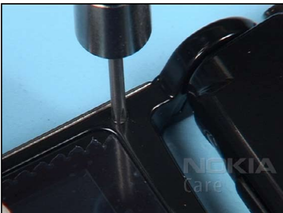
23. Tighten both screws.
