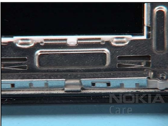
11. Note the correct positioning and click the snaps into their places.
