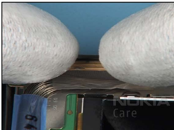
13. Align the coax cable and close the connector.
