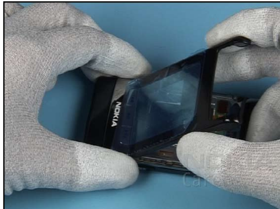
8. Lift up and remove the A-COVER.
