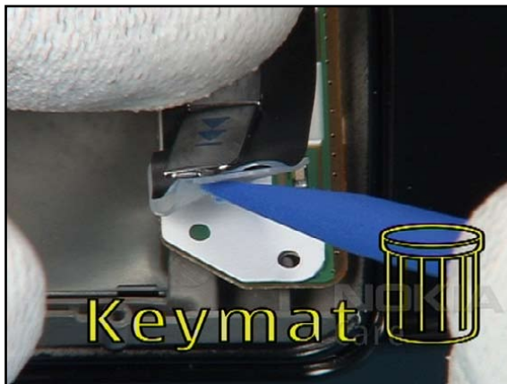
20. Gently peel of the MEDIA KEYMAT. Remove the adhesive residues.
