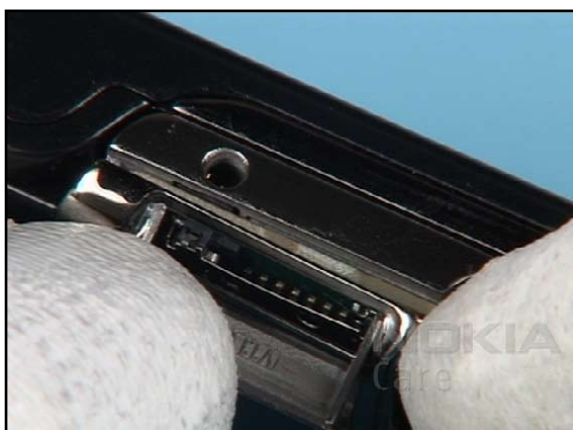
11. Move the left tab of the SD DOOR to the recess of the D-COVER.
