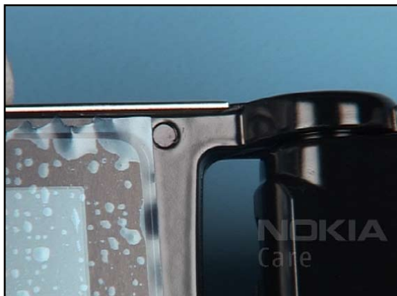
24. Cover the screws with new SCREW CAPS.
