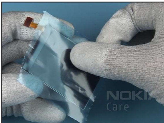
23. Cover the display with a protective film.
