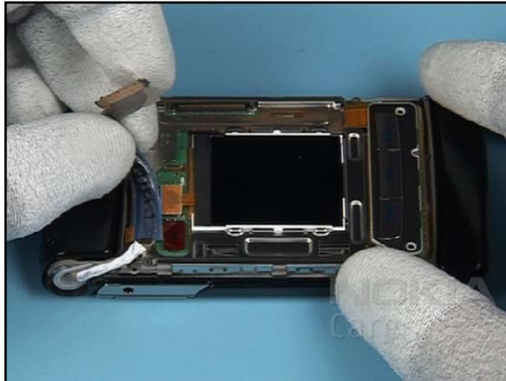
14. The coax cable is glued to the LID FRAME.
