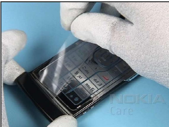
35. Remove the protective film.
