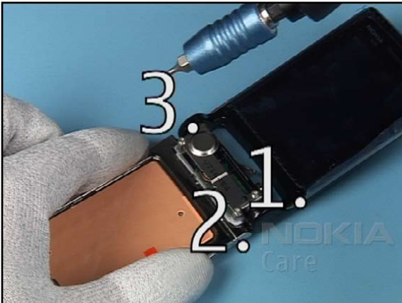
25. Unscrew the 3 screws in the order shown and discard them.
