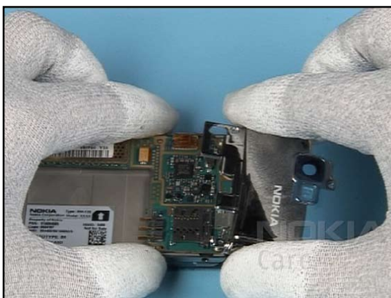
22. Place the D-COVER over the engine module.
