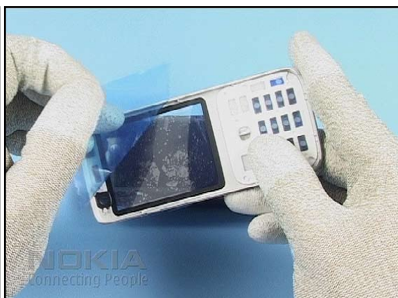
42. Check the window for cleanliness ...
