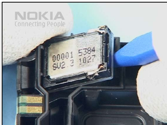
40. Lift the IHF SPEAKER from its housing and remove it easily.
