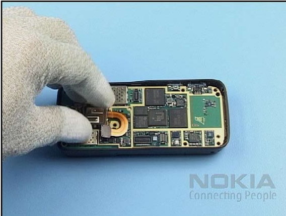
19. Insert the MAIN CAMERA into its housing...
