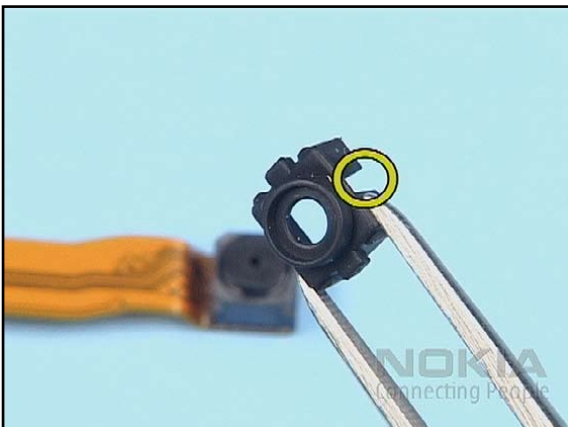
23. Ensure the correct position of the CAMERA BOOT when putting it onto the FRONT CAMERA.
