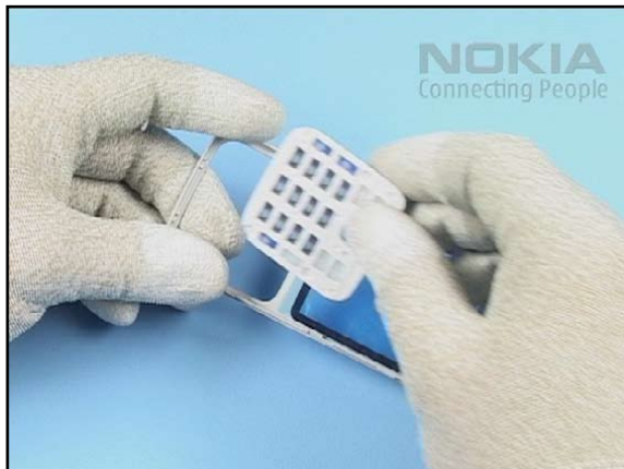
12. Unlock and remove the KEYMAT.
