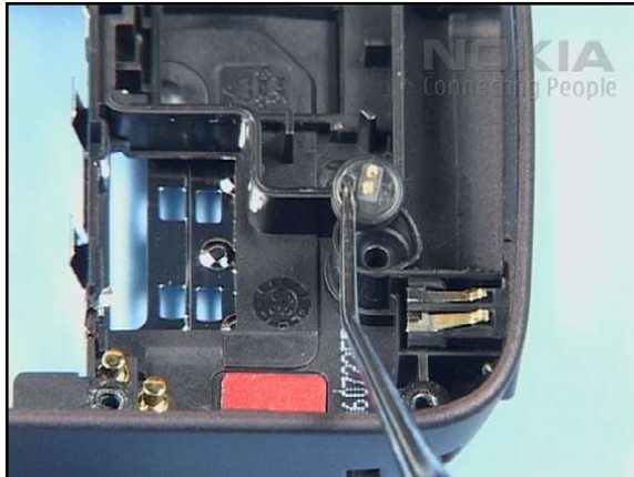
44. Remove the MICROPHONE with the dental pick.
