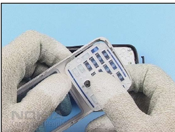
41. Put the KEYMAT into the A-COVER.
