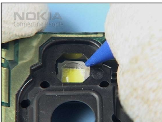
41. Gently push down the FLASH LED from the ANTENNA MOULDING.
