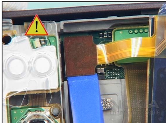
16. ...and disconnect it from the ENGINE MODULE.
