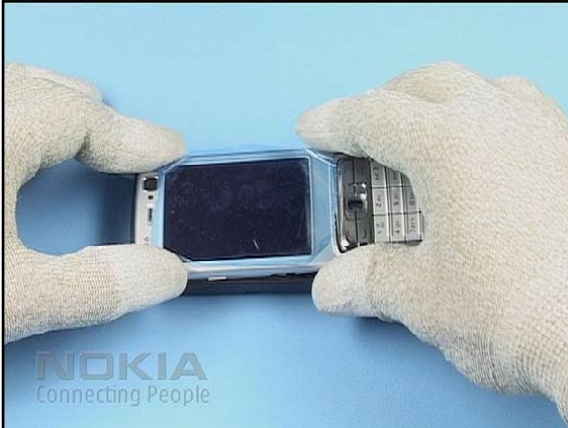
43. ... and fit the A-COVER to the B-COVER.
