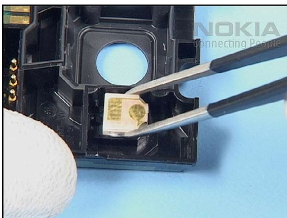
10. Place the FLASH LED into its socket and secure it carefully with the SS-93.
