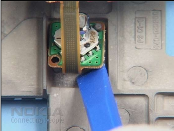
31. Place the UI MODULE over the JOYSTICK HAT and carefully lever out the MODULE from the UI FRAME with SS-93.
