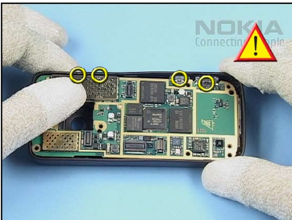
15. Pay special attention to the SWITCHES when inserting the ENGINE MODULE into the B-COVER.
