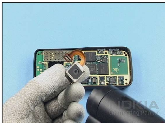
18. and the MAIN CAMERA with compressed air.
