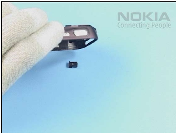
46. The DC-JACK drops out easily when turning the B-COVER.
