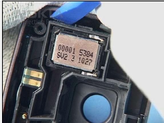
38. Unlock the ANTENNA MODULE ASSEMBLY with the SS-93 ...
