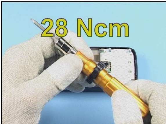
34. Set the torque driver to the torque of 28 Newton centimeter.
