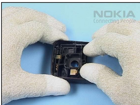
11. Insert the ANTENNA MOULDING in the B-COVER...
