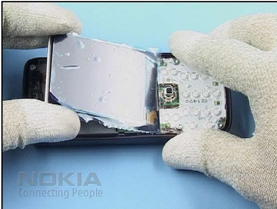
37. ... and place it carefully onto the UI FRAME.
