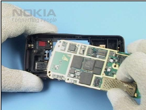
37. ... and remove it as shown taking care to all spring contacts.
