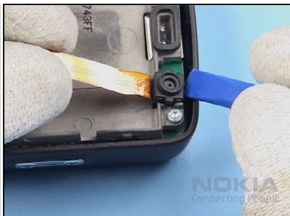
18. Remove the FRONT CAMERA from the UI-FRAME.
