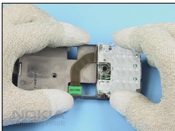
30. Open the snap if it snapped back and remove the LIGHT GUIDE.
