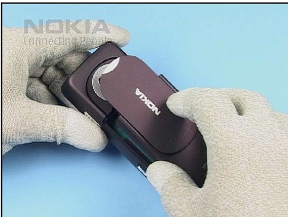
45. Fit the SLIDE COVER ASSEMBLY
