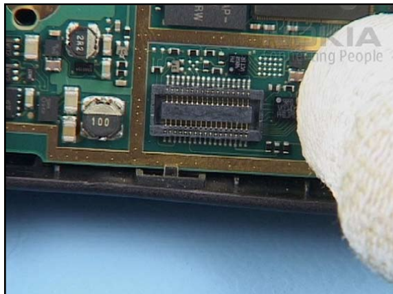
16. Secure the ENGINE MODULE.
