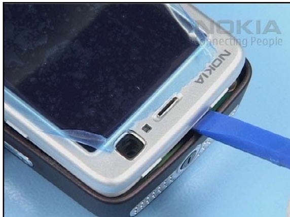
10. Lift the A-COVER a bit and unlock its top side from the B-COVER with the SS-93.
