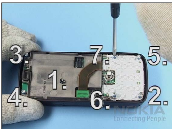
21. Undo the screws in the order shown.
