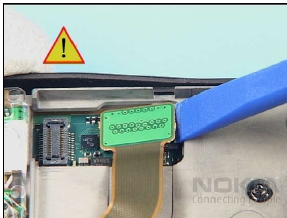
20. Carefully open the UI MODULE connector taking special care to the surrounding components.
