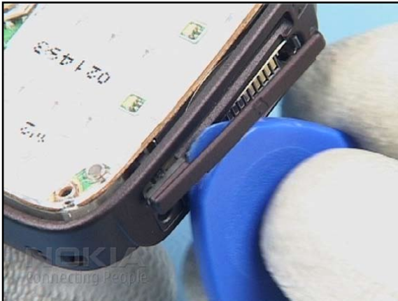
25. Open the SD DOOR but do not remove it yet.
