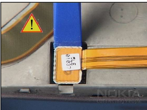
17. Open the FRONT CAMERA connector.
