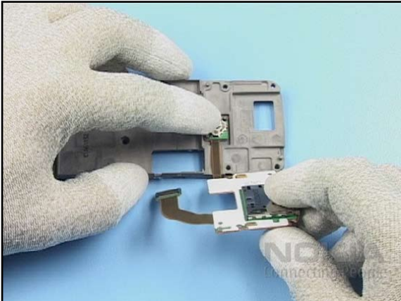
25. Position the UI MODULE onto the UI FRAME and slightly press on the JOYSTICK HAT to ensure that it is glued.
