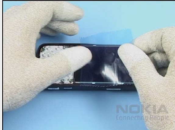
14. Cover the DISPLAY with a protective film.
