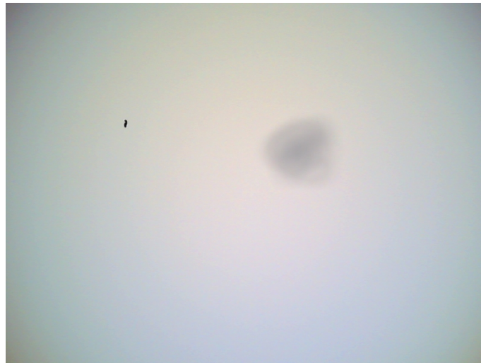
Figure 75 Effects of dust on optical path
