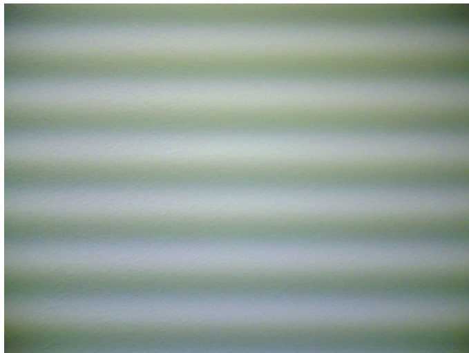
Figure 71 Flicker in an image; object illuminated by strong fluorescent light
