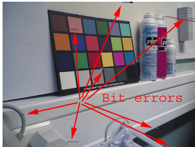
Figure 78 Bit errors caused by JPEG compression
