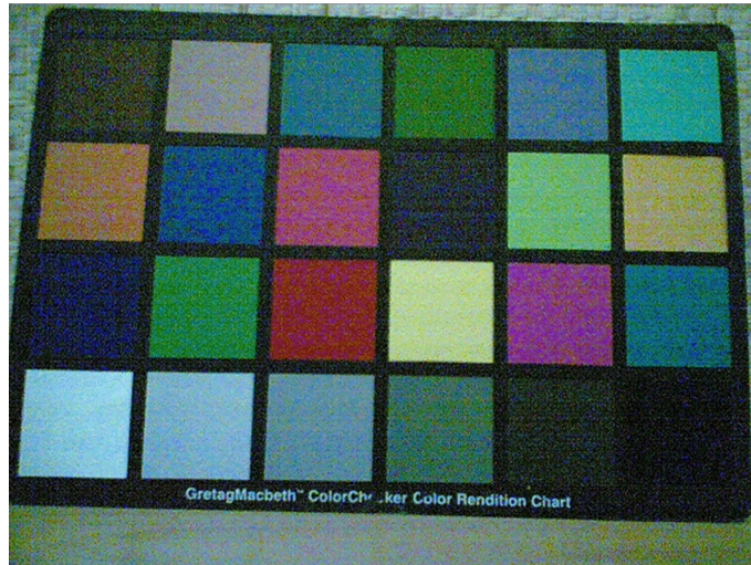
Figure 69 Noisy image taken in +70 degrees Celsius
