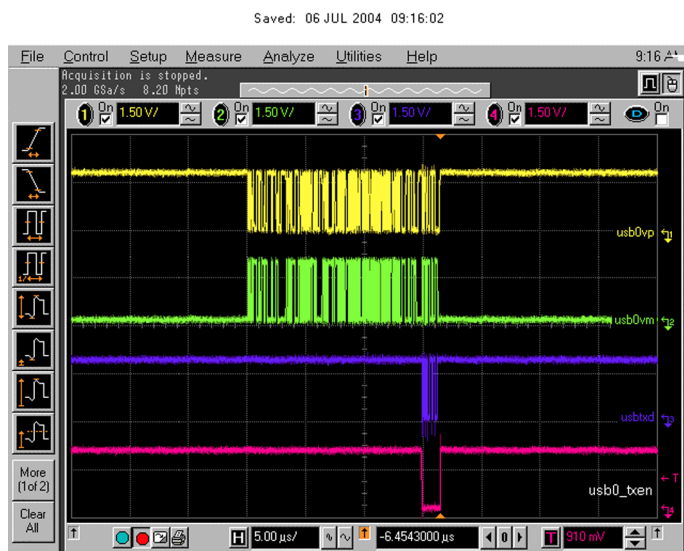
Figure 42 USB 2: Take single triggered measurement on the rising edge of the application processor usb0_txen (J4813) line.
