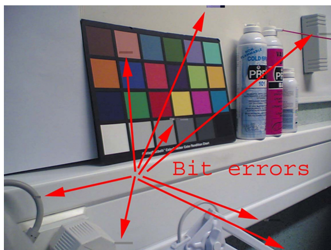
Figure 72 Bit errors caused by JPEG compression
