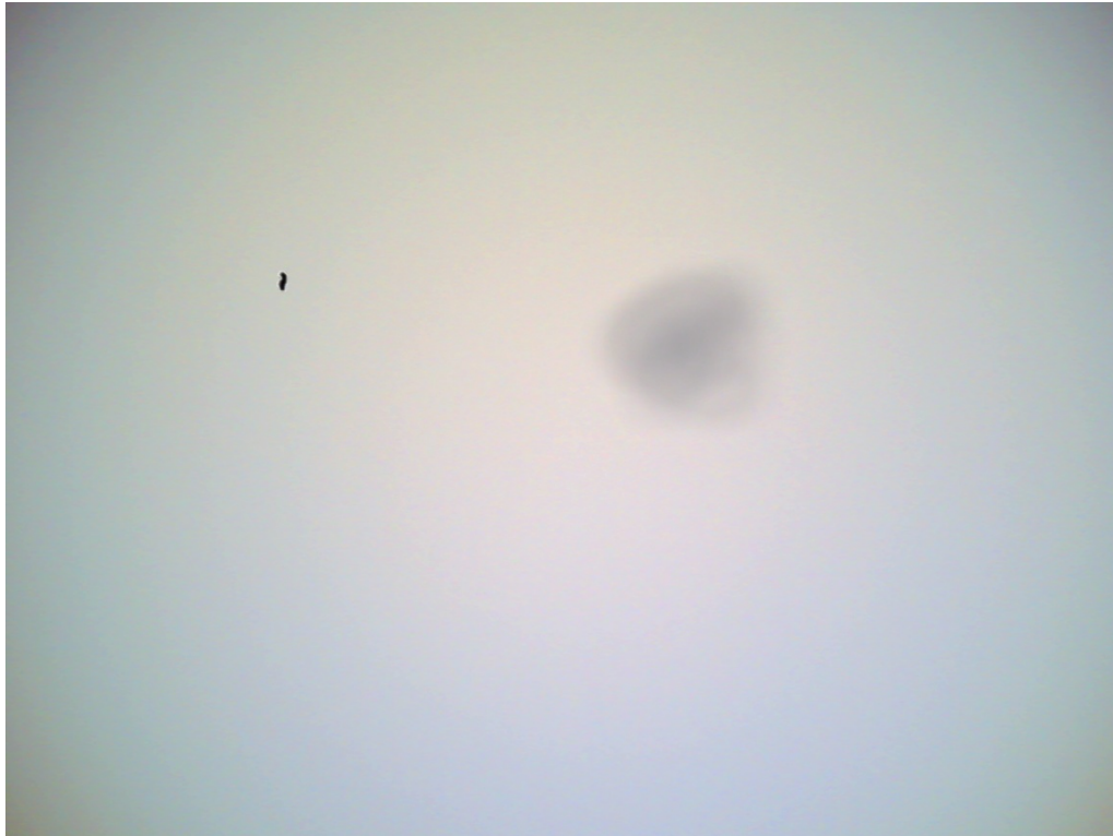
Figure 10 Effects of dust on optical path
