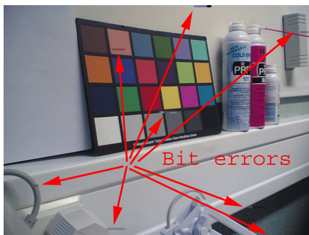
Figure 13 Bit errors caused by JPEG compression
