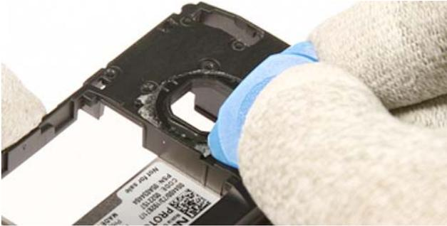
33.) Remove the residues of the **Camera Rear Bezel Assy Adhesive** completely with the SRT-6.
