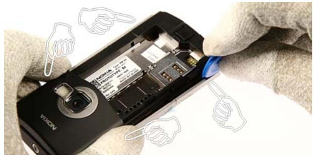
4.) Place the SRT-6 between the **A-Cover** and **Chassis Assy**. Release the 4 plastic clips beginning from the bottom side as shown.
