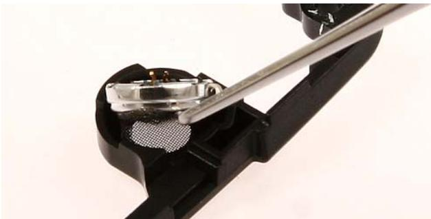
19.) Remove the **Earpiece** with the dental tool
