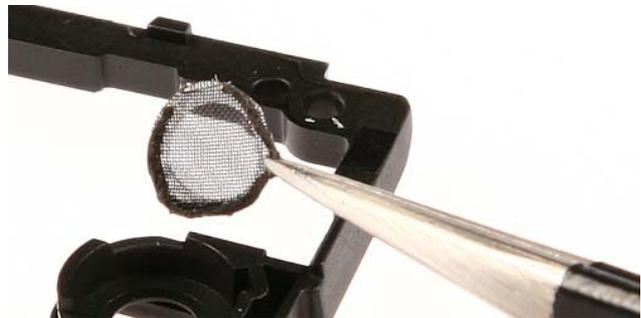
20.) Also remove the **Earpiece Gasket** from its compartment. **Always use a new gasket when reassembling.**
