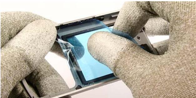
7.) Also protect the inner side window with a film
