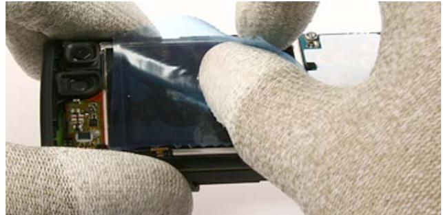
6.) Protect the **LCD** with a plastic film.
