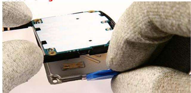
22.) Then push down and remove the **BB Shield Assembly**. The shield can't be reused again, always use a new one.
